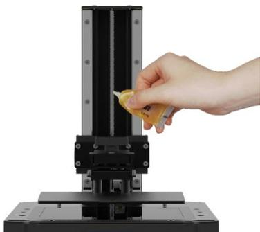
(1) If Z axis make noisy sound, please apply lubricant to Z lead screw.
