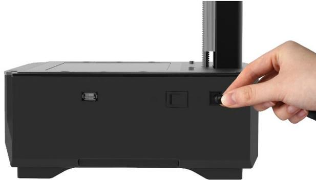
2. Raise Z axis to a certain height that the LCD screen will not be scratched when the printing platform is installed.
