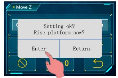
9. Detection: Raise printing platform until the curing screen can be observed completely. Return to Tools menu and click "Detection". Set the test time and then click "Next". The curing screen should display a complete image as shown below.
