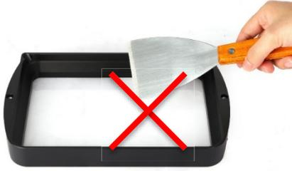
(2) Remove the cured resin from release film: Set full-screen exposure for 20s and then remove the cured resin sheet to protect the film. **DO NOT use sharp objects to scrape off the residues on FEP film.**
